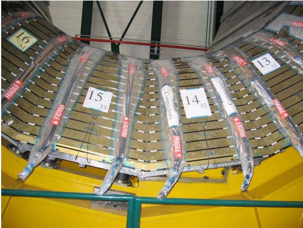
Figure 5.8: Close up view of the assembled HB wedges, showing the optical cabling.
