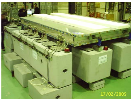
Figure 7.24: The chamber calibration bench in the CERN ISR Lab.
