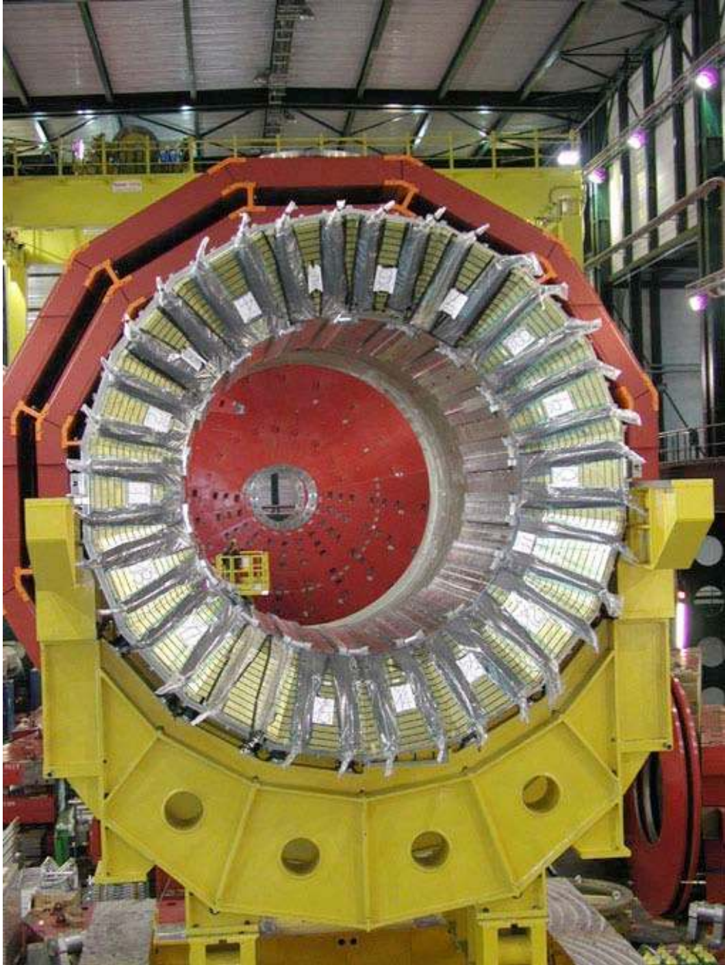
Figure 5.2: Assembled HCAL half-barrel in SX5, the above ground assembly hall.
