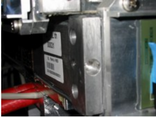
Figure 7.11: Corner blocks of an SL. These pieces also carry the reference marks with respect to which the wire positions are measured.
