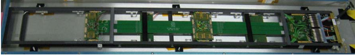
Figure 3.27: Photo of a rod frame equipped with electronics components, ready to receive silicon detector modules.
