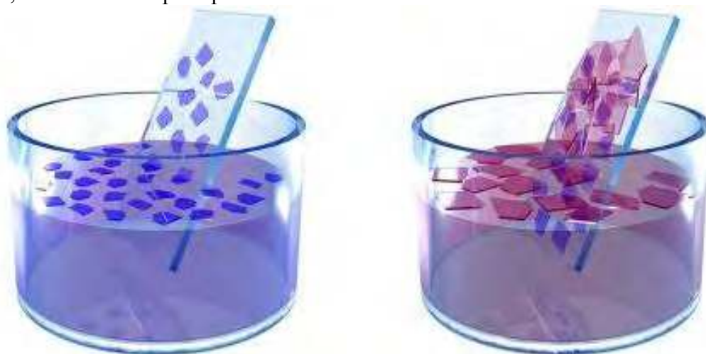
Fig. 52 Superstructure assembly by dispersions and inks. In the example reported in figure, a dip casting strategy is used to deposit successive layers of different 2d crystals to create an heterostructure.
