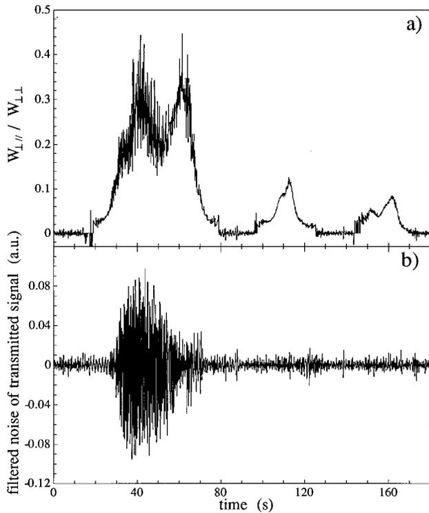
FIG. 5. Time development of (a) the  $W_{\parallel}/W_{\perp}$  ratio and (b) the level of the low-frequency noise filtered out of the transmitted signal. Plasma parameters: 15.4 sccm silane at 0.20 mbar, rf power 3.3 W at 13.56 MHz, reactor and electrodes at room temperature.
