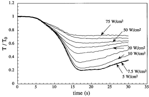
FIG. 2. Time evolution of the normalized transmitted intensity of the laser beam  $T/T_0$  for different incident laser fluences at the plasma. Plasma ignition at time = 0 s. Plasma parameters: 7.7 sccm silane at 0.25 mbar, rf plasma power 2.9 W at 13.56 MHz, reactor and electrodes at room temperature.  $\text{Ar}^+$  laser at 488 nm wavelength, positioned 5 mm above the lower electrode and displaced by 29 mm towards the detectors from the electrode axis.
