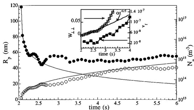
FIG. 6. Time development of the particle radius  $R_p$  (○), and the number density  $N_p$  (●) for early discharge times (Rayleigh scattering). Solid lines show the best fit of the Brownian free molecule coagulation model ( $R_c=2.4$  nm and  $N_c=4 \times 10^{17} \text{ m}^{-3}$ ). The inset presents the first second of the scattered light time evolution (□) and  $t^{6/5}$  time dependence fit and the volume fraction  $v_f$  (■). Plasma parameters and laser position as for Fig. 2.
