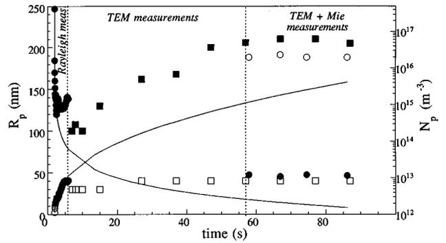
FIG. 7. Time development of the particle radius  $R_p$  (○) and the number density  $N_p$  (●), and the lower (□) and the upper limit (■) of particle radius obtained from the TEM measurements. Solid lines fit from the Brownian free molecule coagulation model as in Fig. 6. Plasma parameters and laser position as for Fig. 2.
