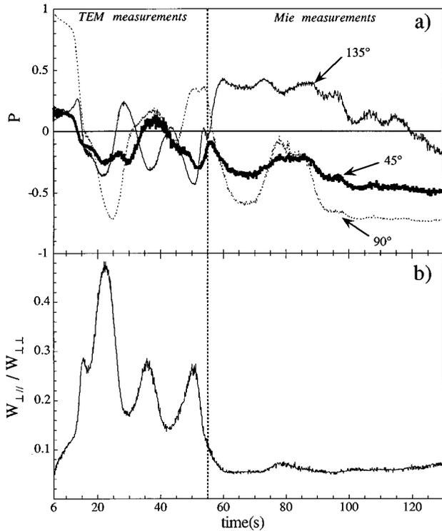
FIG. 3. Time development of (a) the linear polarization degree,  $P$ , at 45°, 90°, and 135°, and (b) of the cross-polarization intensity normalized to the corresponding direct polarization  $W_{\perp\parallel}/W_{\perp\perp}$  at 135°. Plasma parameters and laser position as for Fig. 2, with a laser intensity of 5 W/cm<sup>2</sup>.
