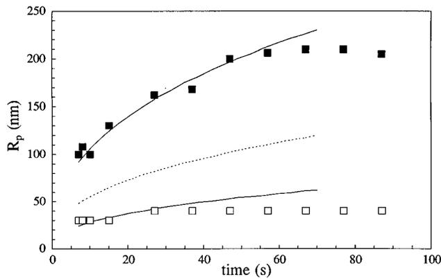
FIG. 9. Comparison between the particle radius distribution measured from the TEM measurements, the lower ( $\square$ ) and the upper limit ( $\blacksquare$ ), and calculated from Brownian free molecular coagulation model with self-preserving log-normal distribution. Dashed lines represent the particle radius at the maximum and solid lines at 10% of the maximum of the log-normal distribution.
