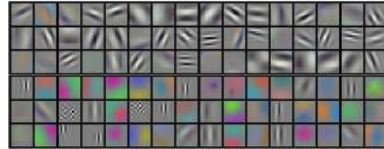
Figure 3: 96 convolutional kernels of size 11 \times 11 \times 3 learned by the first convolutional layer on the 224 \times 224 \times 3 input images. The top 48 kernels were learned on GPU 1 while the bottom 48 kernels were learned on GPU 2. See Section 6.1 for details.
